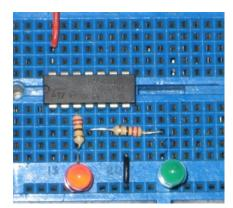
An LED almost always has a series resistor.
