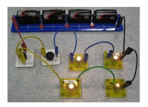
Ammeters and voltmeters are always added to the circuit after it has been built and tested - these are measuring instruments and should not actually affect the working of the circuit.
