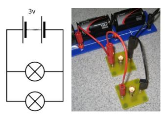
Adding components in parallel simply involves connecting each end of the two components together so that the circuit splits and the current can go down one branch of the circuit or another. Again, keep the layout as close to the circuit diagram as possible and ensure the colour code is consistent. Wires that join should be the same colour therefore only RED and BLACK are used in this circuit.
