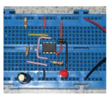
When wiring up an IC always start with the power supply wires so that you don't forget about them later on.
