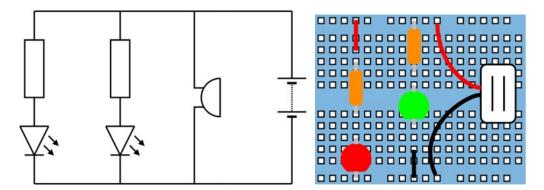
The RED LED and resistor in the circuit are connected using the vertical tracks. Notice how each component crosses a gap between one track and the next and a wire link is needed to make the connection from the positive rail to the resistor.
