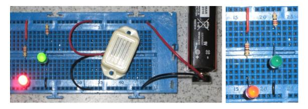
The close up shows the LED connections in detail. A RED wire links from the positive rail, crosses the gap and connects to a spare track. The connections in the protoboard mean the lower end of the RED wire is now connected to the upper end of the resistor. The resistor crosses the central gap and the lower end of the resistor is now connected to the upper end of the LED. The LED bridges the gap at the bottom of the protoboard and connects to the zero volt rail.
