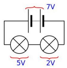
In this case the total EMF is the individual EMF of each cell in the battery which all add up to 7 volts.
