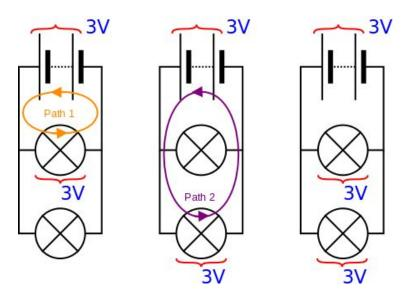
In path 1 in the diagram, the EMF of 3 V is matched by a Pd of 3 V across the first bulb.
