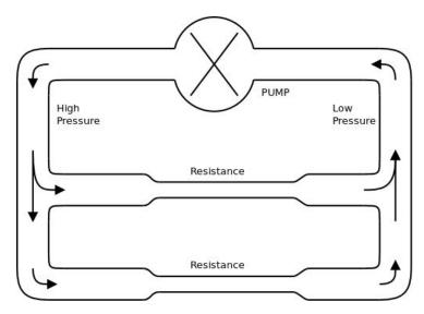
This analogy considers water flowing through pipes to make a water circuit, this is similar to the water circuit in a central heating system.
