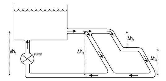
**Analogy:** Water is pumped up to a height gaining potential energy which is analogous to charge carriers going through a cell gaining electrical energy. The height represents the 'voltage'. Water flowing downhill gains kinetic energy but loses height which is analogous to electrical energy being transferred to some other form. Water flowing along a level channel loses no height just as current through a wire does result in a significant potential difference.
