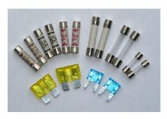
A fuse is a thin piece of wire included in a circuit. The material from which the fuse wire is made usually has a lower melting point and a slightly higher resistance than the other wires in the circuit. If too much current flows in the circuit, the fuse wire will get hot (due to its higher resistance) and melt (due to its lower melting point) before any of the other wires get hot. Once the fuse melts, the circuit is broken and no more current flows.
