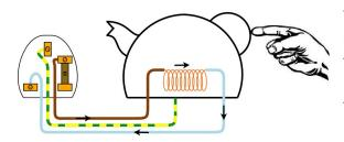
The circuit is working properly, there is no fault. Current flows in the Live and Neutral wires - the element glows. No current flows in the Earth wire, the person is not electrocuted and the fuse doesn't blow.
