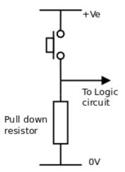
When the push button is not pressed, the logic circuit is connected to 0 V through the resistor. The input to the logic circuit is Logic 0.
