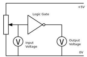
The circuit shown can be used to investigate the exact transition point of a logic gate. The potentiometer provides a variable input voltage and voltmeter measures the input voltage. A second voltmeter measures the output voltage.
