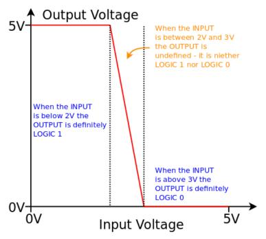
A graph of Input voltage against Output voltage is called the transfer characteristic of the logic gate - it shows how the input and output voltages are related. The diagram shows a typical transfer characteristic for a Logic NOT gate but it should be noted that all logic gates have their own transfer characteristics and, if the exact values are needed, then the logic gate must be tested.
