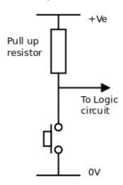
When the push button is not pressed, the logic circuit is connected to positive through the resistor. The input to the logic circuit is Logic 1.
