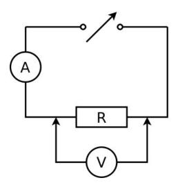
For any resistor, the relationship between voltage and current can be investigated and the nature of the resistor determined by measuring values of potential difference and current using the test circuit shown. These values can be plotted on a graph of current (x-axis) and voltage (y-axis). Alternatively a graph of voltage (x-axis) against current (y-axis) is equally valid - you need to recognise both.
