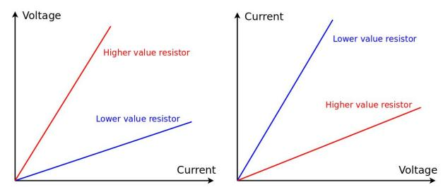
A fixed resistor is a resistor that has a constant resistance. The graph of potential difference against current for a fixed resistor is a straight line.
