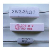
A resistor is a component that opposes the flow of current. In a simple circuit containing a battery and a bulb the battery causes current to flow through the bulb and the bulb has resistance that limits the current that can flow. In the bulb electrical energy is transferred to light and heat. In any resistor electrical energy is transferred to heat.
